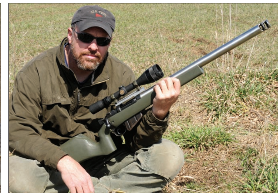
The Lee-Enfield sported a shortened wartime production two-groove barrel dark from cordite inside a StraightJacket, scope mount and a Teludyne stock.
