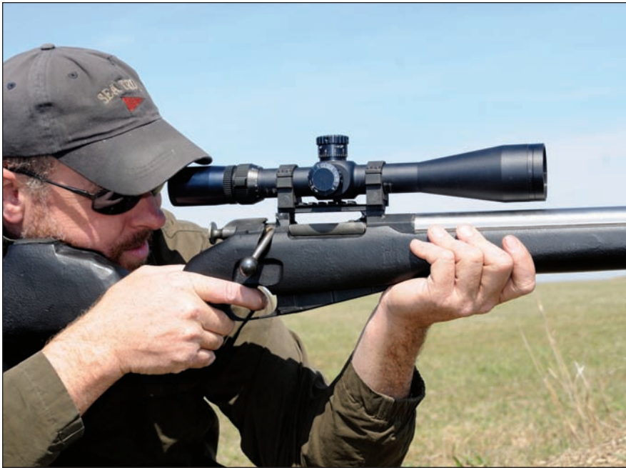
Fortier kicked in a Mosin-Nagant, to which Teludyne added a StraightJacket. TTI added a scope mount, moved the bolt handle and dropped it into a new stock.
