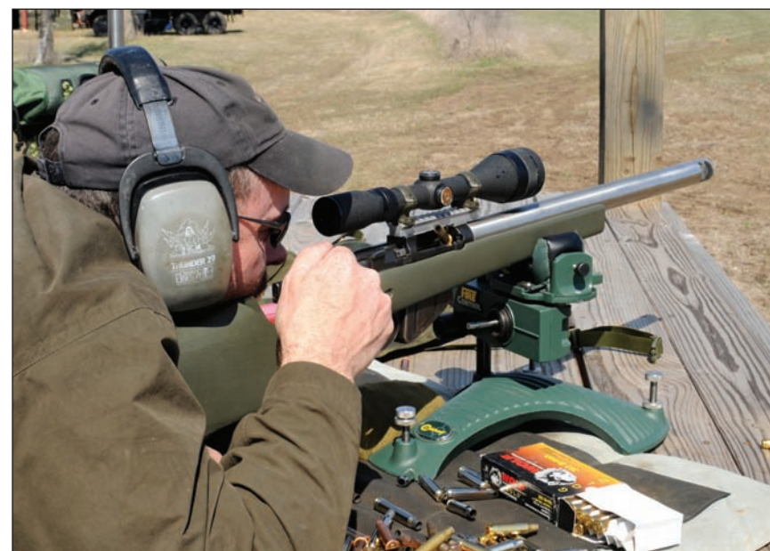
Adolphsen brought a variety of rifles to Fortier's range. Among these was a .303 British Lee-Enfield shop mule. This averaged a respectable 1.5 moa at 500 yards.
