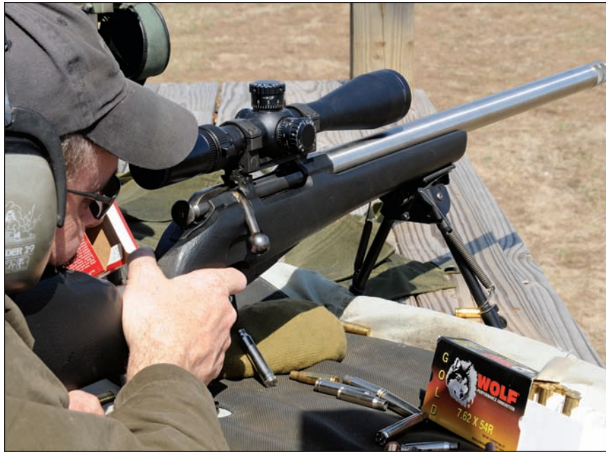
Firing off a bipod, the StraightJacketed Mosin-Nagant averaged a respectable 1.5 moa at 500 yards. The TTI muzzle brake made the rifle much more comfortable.
