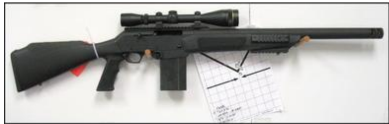
FNAR .308 with StraightJacket installed and the 14 shot group target.
